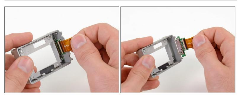
Grasp the SD board ribbon cable gently and pull the SD board out of the rear case.
