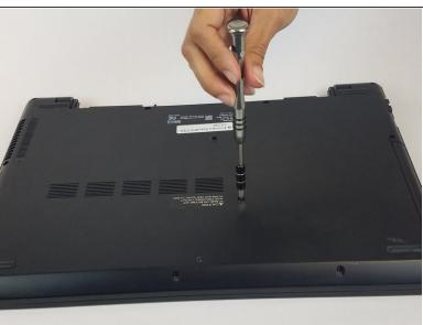
Unscrew the ten 6.5mm PH1 Phillips head screws that hold down the back cover.
