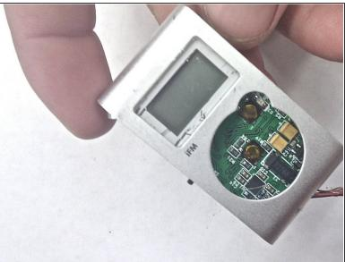
Place the screen cover on top of the LCD so it covers its entirety. Carefully slide the circuit board/LCD back into the device.
