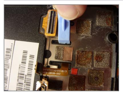
Using a plastic pry tool, lift and remove the three tabs securing the trackpad restrainer to the trackpad.
