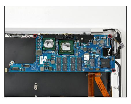
Remove the three Phillips screws securing the logic board to the upper case.
