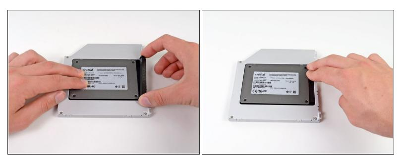
Once the hard drive is snug, reinsert the plastic spacer while holding the hard drive against the bottom of the enclosure.
