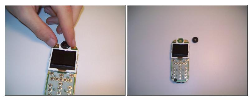
• Lift to remove the speaker from its contact point on the logic board.
