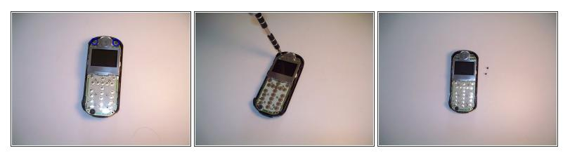
• Using a Torx T-5 screwdriver remove the screws at the top of the phone.
