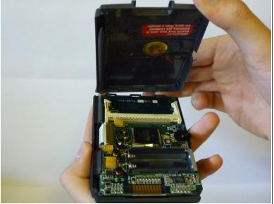
Pull the back cover from the bottom of the device and separate the interlocking tabs on the top to remove the back cover.
