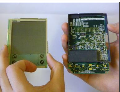
• The screen is now disconnected from the rest of the device and can now be removed.
