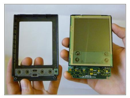
The front plastic cover is now free to be removed from the rest of the device.
