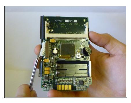
The ribbon cable is now loose. Use the tweezers to carefully slide the ribbon cable out of the connector.
