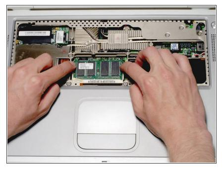
Release the tabs on each side of the RAM chip at the same time. These tabs lock the chip in place and
