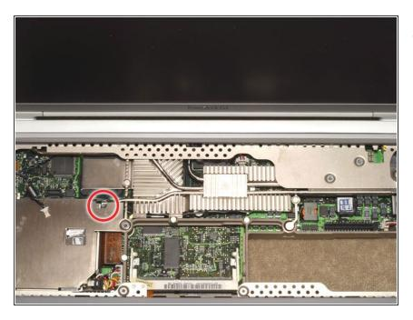
Remove the single T8 Torx screw located near the silver heat pipe.
