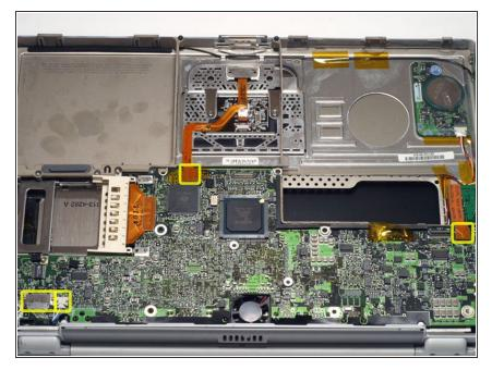
Disconnect the indicated connectors from the logic board, removing tape as necessary.
