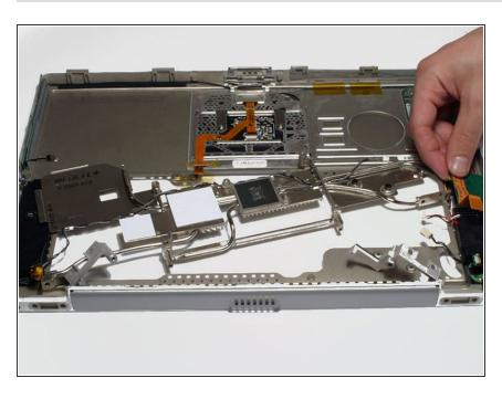
Lift the inverter board out of the computer.
