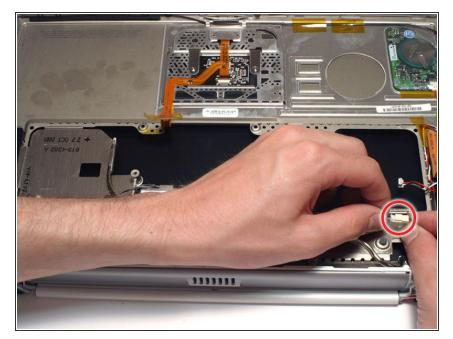
Disconnect the audio cable at the right side of the computer, removing tape as necessary.
