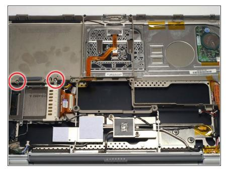
Remove the two T8 Torx screws that secure the PC Card cage.
