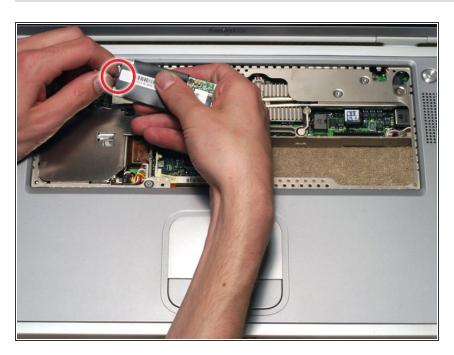
Disconnect the connector cable from the modem.
