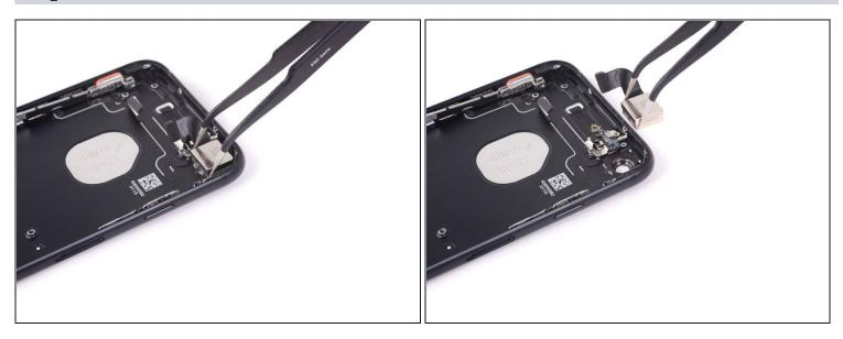
• Use a pair of <u>tweezers</u> to remove the rear-facing camera.
