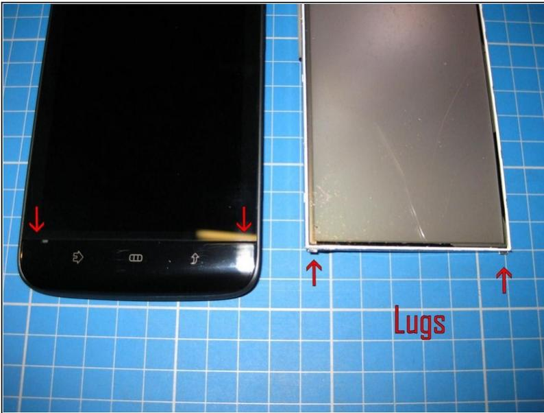
⚠ Here you can see the lugs which hook in the bottom of the chassis to hold the screen in place.
