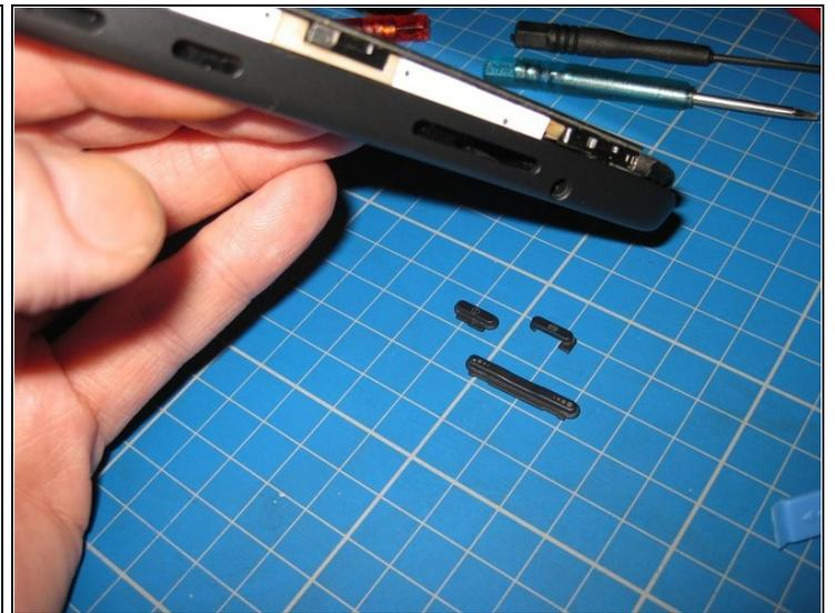
⚠ Note that the side buttons will drop into the case ,so be careful not to lose them also remember the orientation or the buttons! A tip here would be to use some masking tape to hold the buttons in place.
