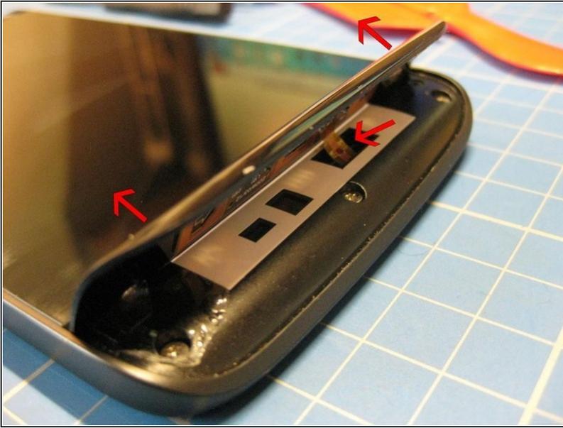
⚠ One thing to be aware of when undertaking work such as this is to ground yourself at the start and regularly through out the operation to avoid any build up of static damaging components. In an ideal world we would all have [Anti-Static wrist straps](#) and work mats, as this is not the case touch a radiator or PC case to dispel any static. Lever up the front edge on the bottom cover be careful not to over extend it due to the ribbon cable to the right side middle.
