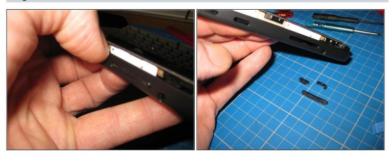
⚠ Note that the side buttons will drop into the case ,so be careful not to lose them also remember the orientation or the bottons! A tip here would be to use some masking tape to hold the buttons in place.
