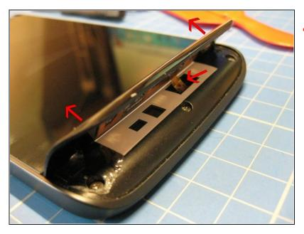
$\triangle$  One thing to be aware of when undertaking work such as this is to ground yourself at the start and regularly through out the operation to avoid any build up of static damaging components. In an ideal world we would all have **Anti-Static** wrist straps and work mats, as this is not the case touch a radiator or PC case to dispel any static. Lever up the front edge on the bottom cover be careful not to over extend it due to the ribbon cable to the right side middle.
