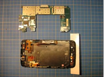
• After following the picture the Logic board should just drop out .There are a few sticky pads under the prying area so a bit of force is needed.
