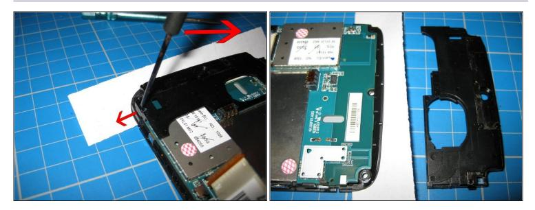
• Using a small flat screwdriver pop this side first! then lift plastic up to the opposite side.
