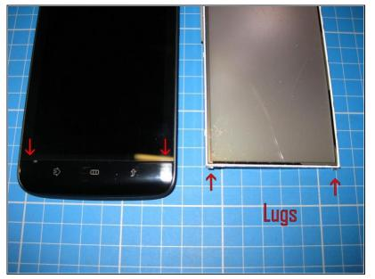
A Here you can see the lugs which hook in the bottom of the chassis to hold the screen in place.
