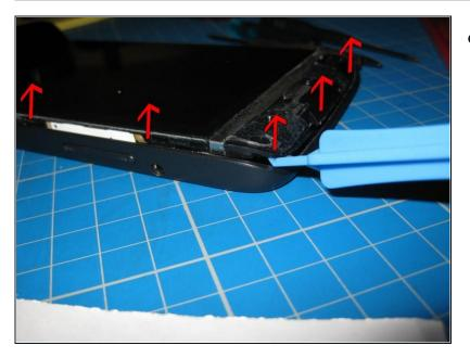
Use a combination of plastic pry and fingernails to work round the edge to lift it.
