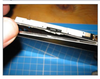
You have to pry the LCD out of the frame of the Streak, it is held in with a strip of gum on either side. A tip here is to start at the top of the phones LCD edge as the bottom of the LCD panel has a couple of lugs which slide into the bottom to lock it in place. More than likely the Gorilla glass will separate from the LCD taking the digitizer with it this is ok.
