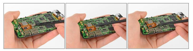
Use the flat end of a spudger to pry the three display cable connectors off their sockets on the motherboard.
