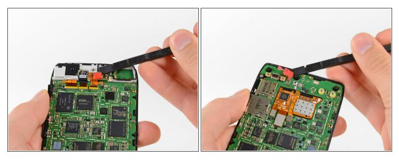
Use the flat end of a spudger to remove the two red silicone microphone covers at the top and bottom of the motherboard.
