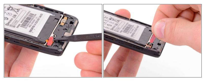
Use the tip of a spudger to lift up the red silicone cover over the battery terminal screws and remove it.
