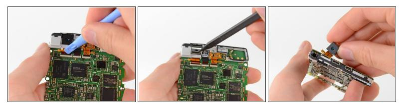
Use a plastic opening tool or your fingernail to lift up the tab on the rear-facing camera ribbon cable ZIF connector.
