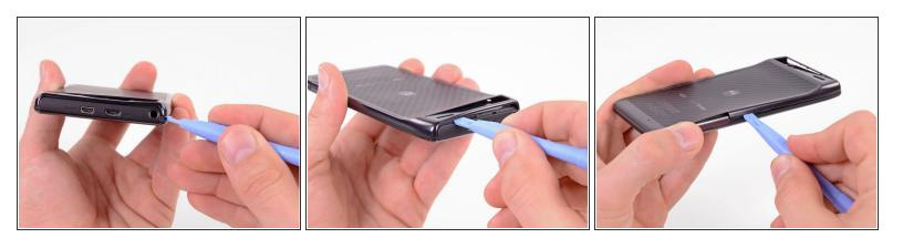
• Work the plastic opening tool across the top of the back case to free the plastic clips.
