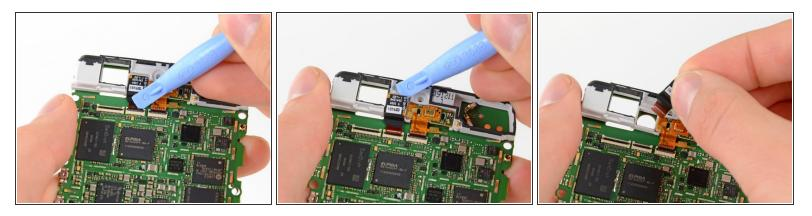
Use a plastic opening tool or your fingernail to lift up the tab on the front-facing camera ribbon cable ZIF connector.
