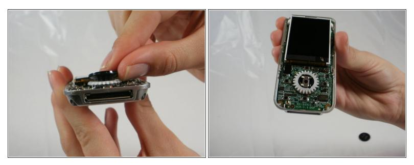
• Gently pry the bottom of the black button to remove it from the device.
