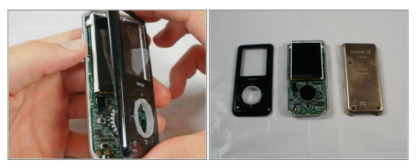
• Pull the front cover away from the rest of the device.
