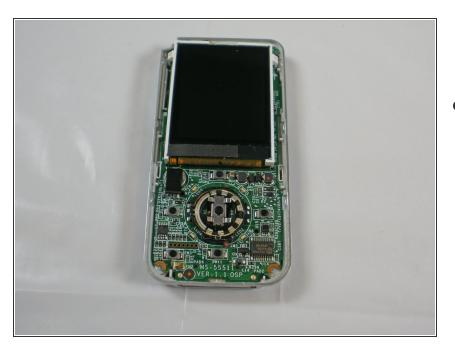
Clean the area around the button to remove any dirt or other outside material that would prevent the scroll wheel from moving freely.
