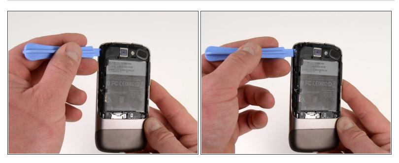
Pry the upper left tab open on the battery housing.
