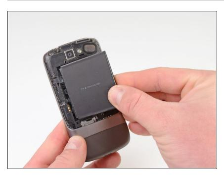
Pull the battery up and out.
