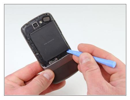
Using the plastic opening tools, pry the left bottom corner of the battery up.
