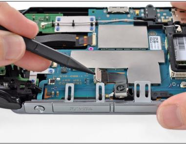
Release the camera flex cable socket by prying up on the tab with a spudger. Leave the socket open.
