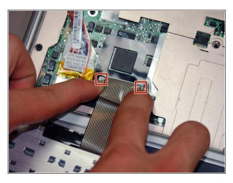
Unlock the ZIF connector on the computer by pushing the two outside tabs toward the screen.
