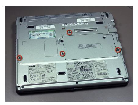
Remove the four 4 mm Phillips #0 screws from the bottom of the laptop.
