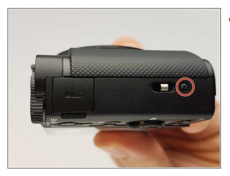
Remove the marked screw with a Phillips #000 screwdriver.
