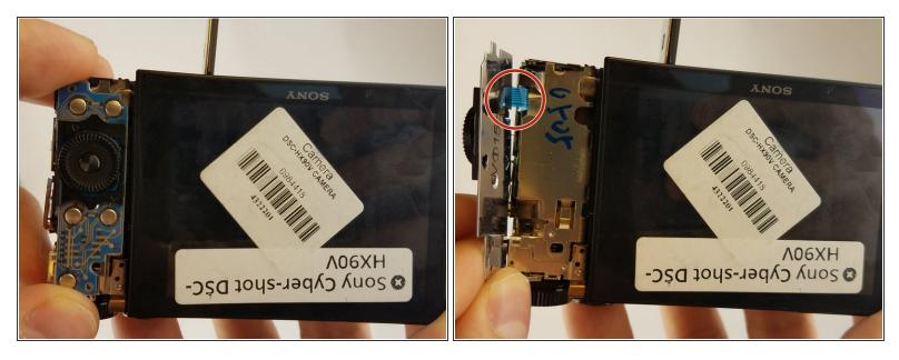
Disconnect the control board data cable with care. Permanent damage may occur to the control board if tools are used to disconnect the data cable. Use your fingers only.
