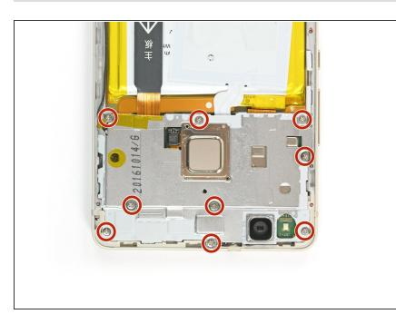
Remove the nine Phillips #00 screws that secure the metal shield plate.
