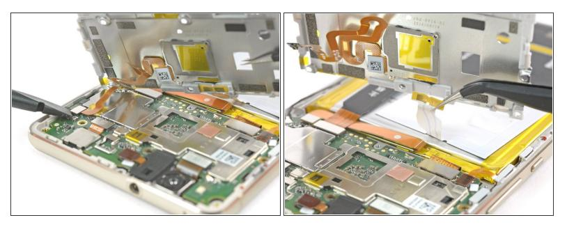
⚠️ Do not remove the shield plate yet, it is attached by a connector and an adhered cable.
