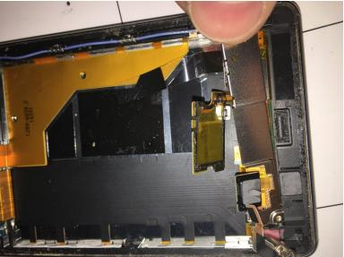
Remove the copper foil, bend the microphone backwards and remove the alluminium shield.
