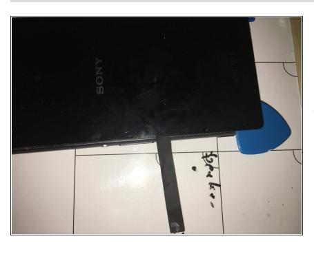
With a pair of tweezers, you should be able to pull out two black tabs. As soon as you can grab them, pull strongly. Then, similar to the iPhone 6, the glue dissolves and you should be able to lift the cover up and away.
