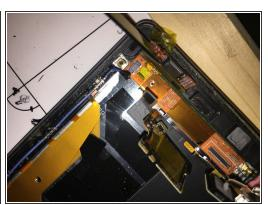
Disconnect the next ribbon. To do that remove the yellow foil and take out the silver plate.
