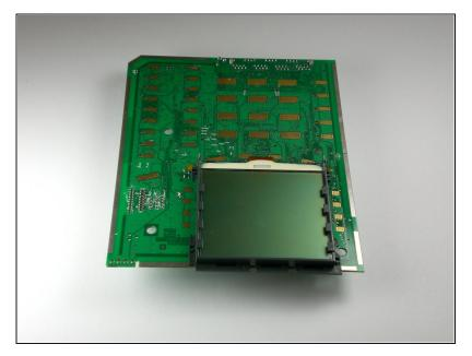
Flip the motherboard over so that the LCD screen is facing upward.
