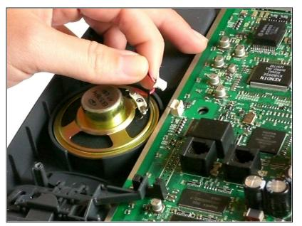
While holding down the motherboard, gently pull the wire harness connecting the speaker to the motherboard until it comes free.
