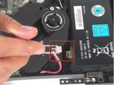
• Remove the white and red wires from the battery by pulling on the base with tweezers.
