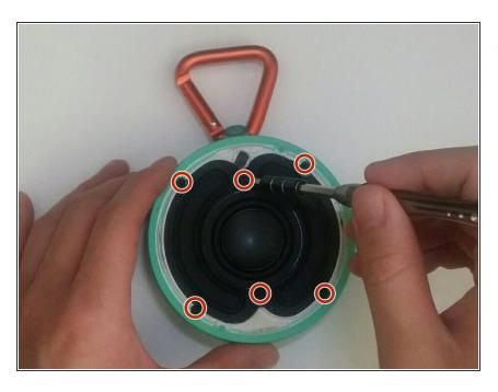
There will be six 3 mm T8 screws under the cap, remove these six screws.
