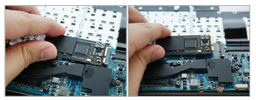
Using your hand, pull the SSD out from its slot.
