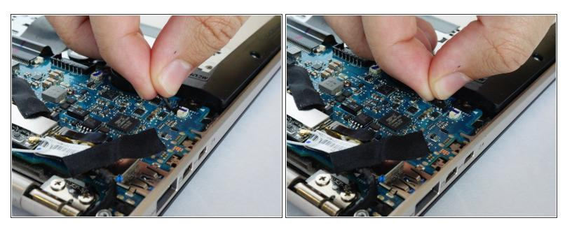
Disconnect the sound cable from the motherboard.
