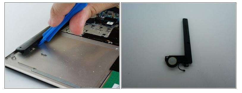
Using the plastic opening tool, pry open the speaker component from the computer.
