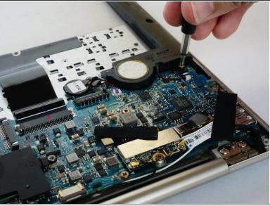
• Remove the screw connecting the speaker component to the motherboard using the screwdriver.
