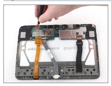
Use a Phillips #000 screwdriver to remove the 3mm screw attaching the motherboard to the display chassis.
