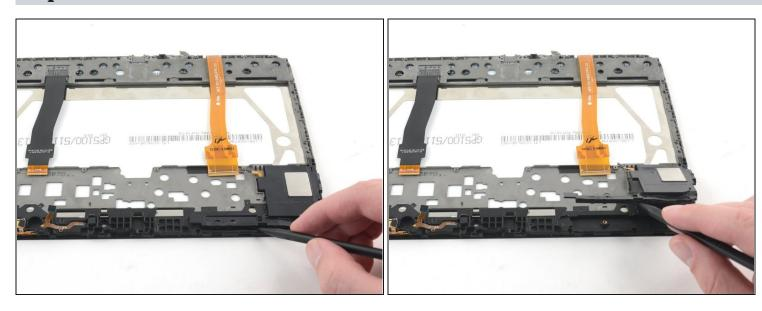
• Use the pointed end of a spudger to pry upwards between the other speaker unit and the display chassis.
