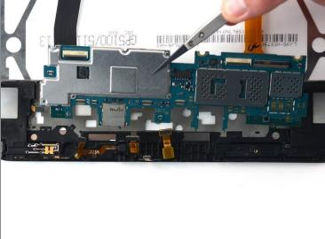
• Use nylon-tipped <u>tweezers</u> to remove the motherboard.
