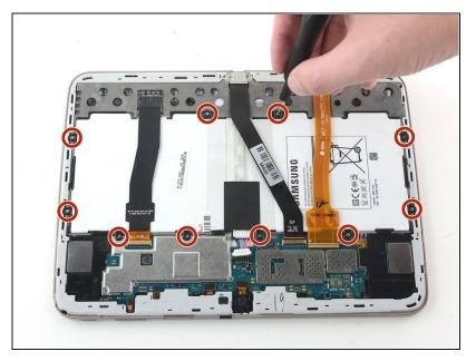
Use a Phillips #000 screwdriver to remove the ten 3mm screws securing the battery to the chassis.
