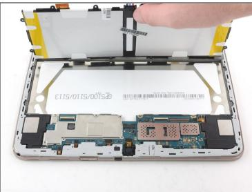
Lift with a nylon spudger to remove the battery.
