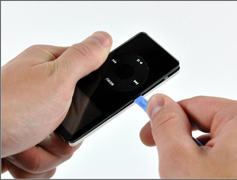
① The large iPod opening tool is no longer needed to gain access to the left side of the iPod.
