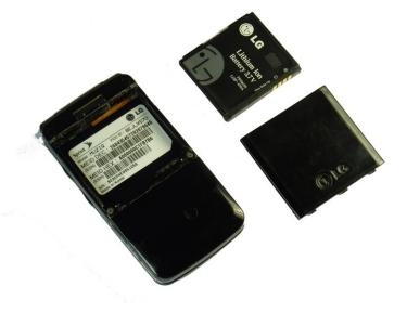
Place a finger at the top corner of the battery and lift out of the phone.
