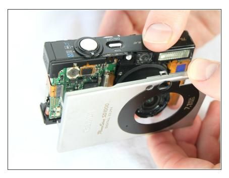
Remove the front cover by gently pulling it away from the camera body.
