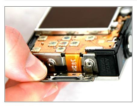
Remove the small cover panel and the attached wrist strap mount.
