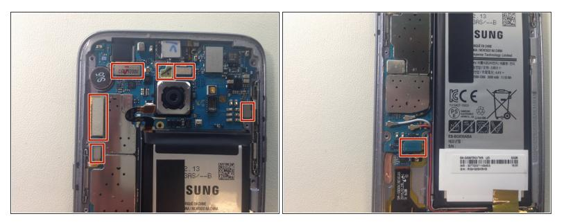
Disconnect all other flex cables connected to the top of the logic board using the flat end of a plastic spudger.
