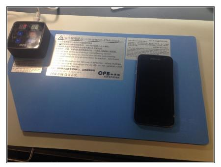
Heat the back of the phone to melt the adhesive holding the back plate on. I use an electronic heating pad, set to 60° Celsius. You can also use a heat gun, but I do not like using them. Be extra careful if using a heat gun, as they are easier to burn yourself with, and holding one over a phone for even just a little too long can damage it.
