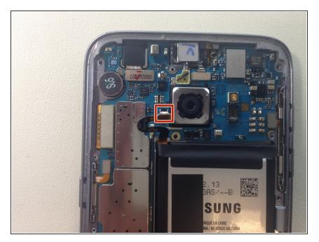
Using the flat end of a spudger, disconnect the battery from the logic board.
