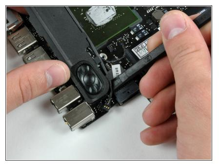
Use the flat end of a spudger to separate the adhesive securing the left speaker assembly to the logic board.
