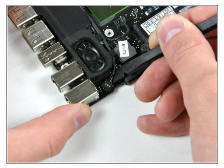
• Use the flat end of a spudger to pry the microphone connector up off the logic board.
