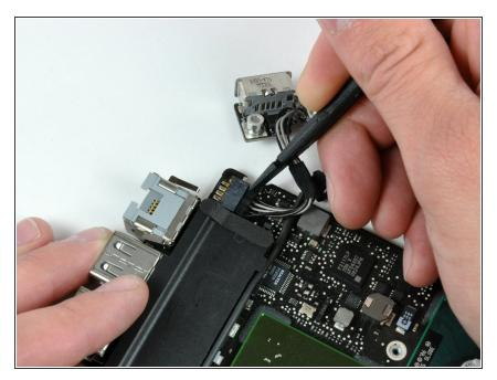
Disconnect the DC-In Board from the logic board by pulling its connector straight away from the socket on the logic board.
