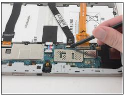
• Use the flat end of a nlyon spudger to pry up the **black** plastic tabs securing the two ZIF connectors.
