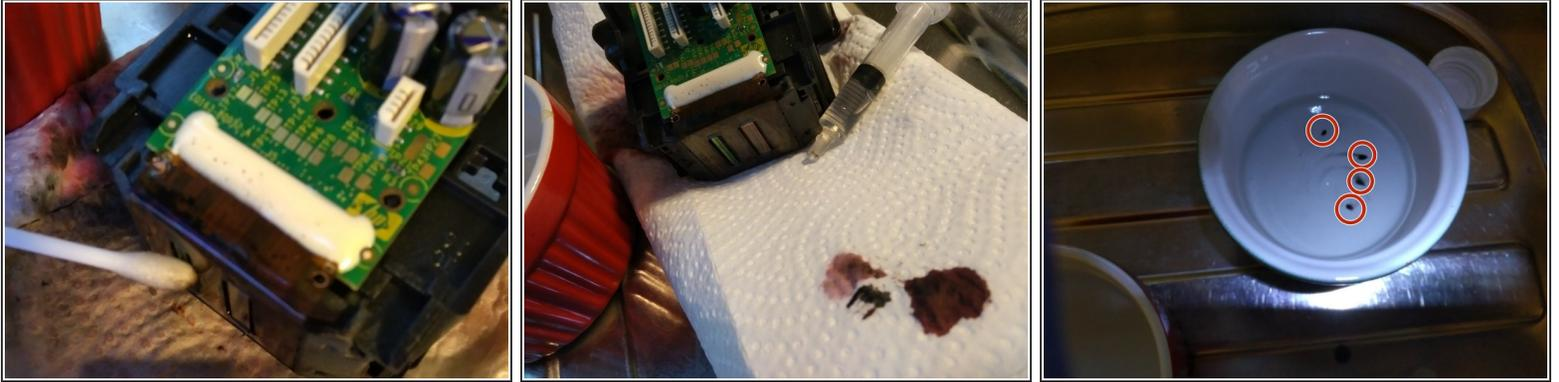
**i** Please note: It is important that you do not spill distilled water or regular water on the PCB. Use a cotton swab to clean around the PCB.
