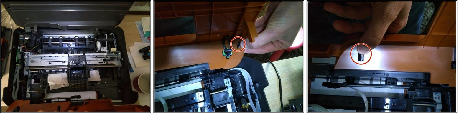
**⚠** Next, remove the orange cover. Use caution as the display unit is still attached to the cover. If you pull the cover off too quickly, you could tear the flat cable.
