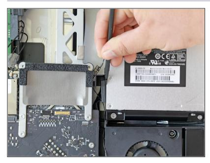
• Use the flat end of a spudger to pull the optical drive data cable out of the optical drive.
