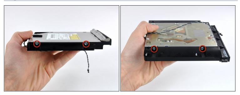
• Remove the two T10 Torx screws from each side of the optical drive (four screws total).
