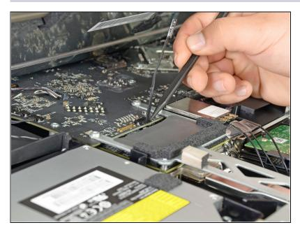
• Use the tip of a spudger to disconnect the display power cable next to the display data cable.
