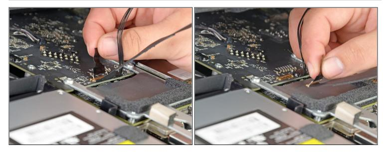
• Pull the black tab straight up to disconnect the latch on the display data cable ZIF connector.
