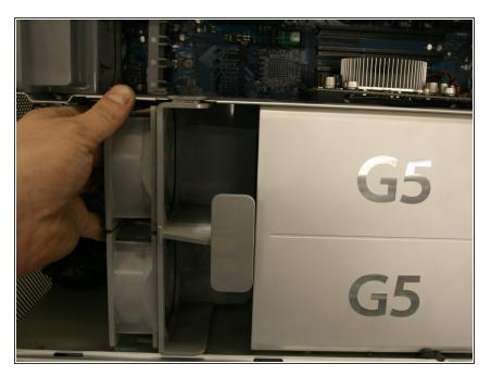
Remove the major fan located on the left side of the processor
