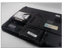
Pull the black ribbon back and up to remove the Hard Drive.
