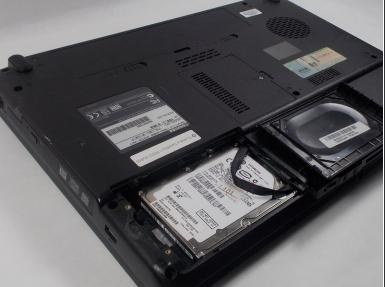
Remove the cover to reveal the hard drive.
