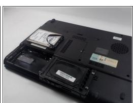
• Pull out the hard drive using the ribbon attached to it.
