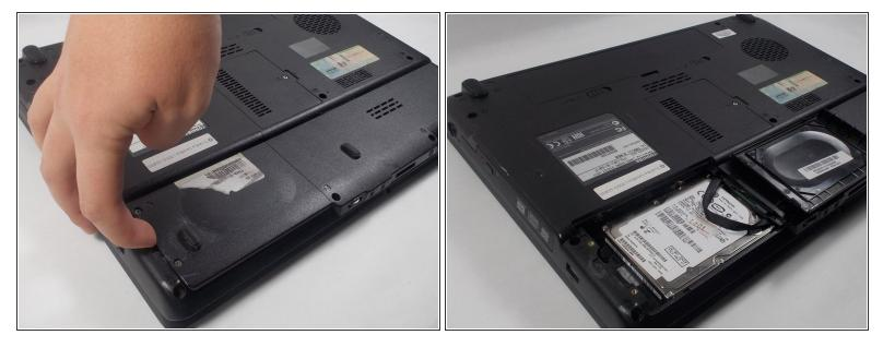
Use your finger to lift and remove the cover to the Hard Drive.
