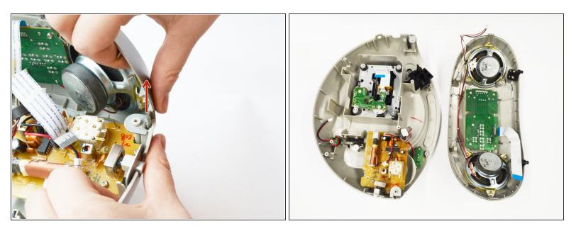
• After the screws are removed, the front can be removed by pulling it upwards.
