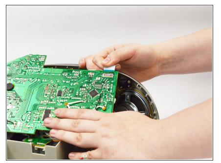
Then the PCB is only connected with these flat white wires. They can be detached by softly pulling on them.
