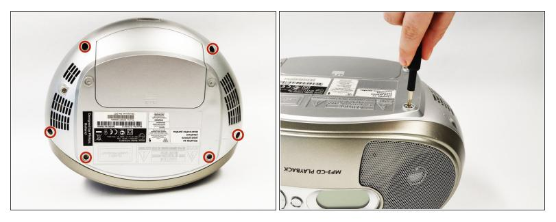
A Take the radio off the net (remove the power cable) and remove the batteries if necessary
