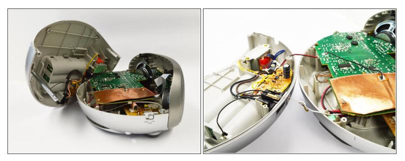
• The bottom can be removed. Attention: the bottom of the radio is still connected to the upper part because of two connections between the PCB's.
