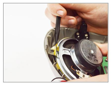
Right now, the speaker is only attached by glue. Remove the glue by using something sharp, like a spudger, to break it.
