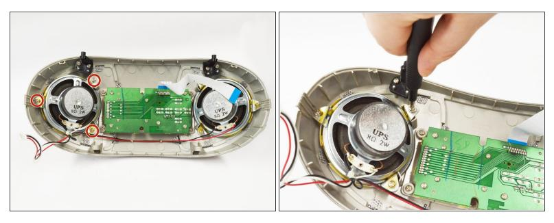
• The speaker is screwed to the front of the casing with three 12.1mm Phillips #0 screws, as can be seen in the picture. Remove these screws with a Phillips 00 screwdriver.
