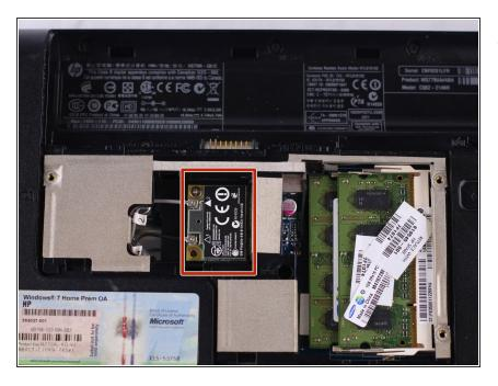
Locate the the Wireless Card located next to the RAM chips.
