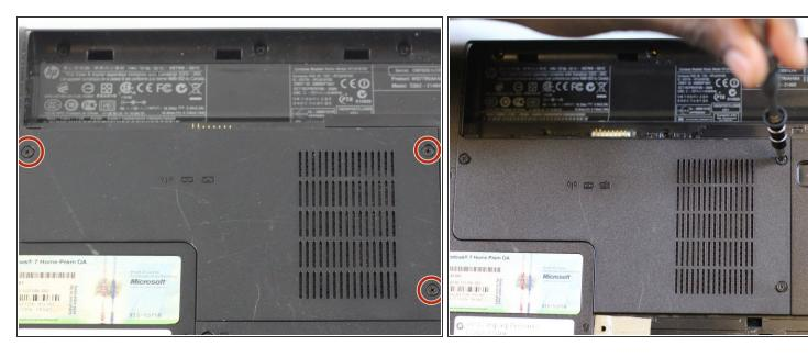
Remove the three M2.5x5 mm Phillips screws securing the memory case.
