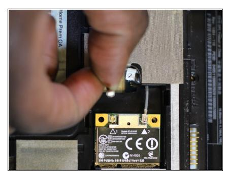
Using your hands, gently remove the cables connected to the wireless card.
