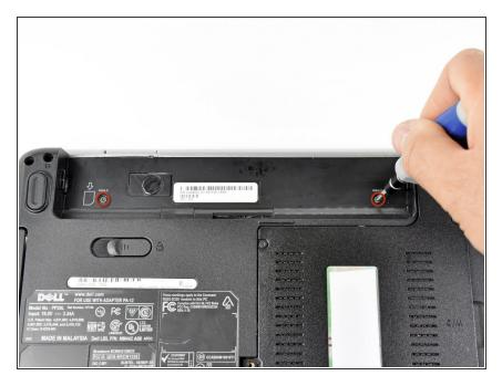
Remove the two 4.00 mm Phillips #1 screws from the battery tray.
