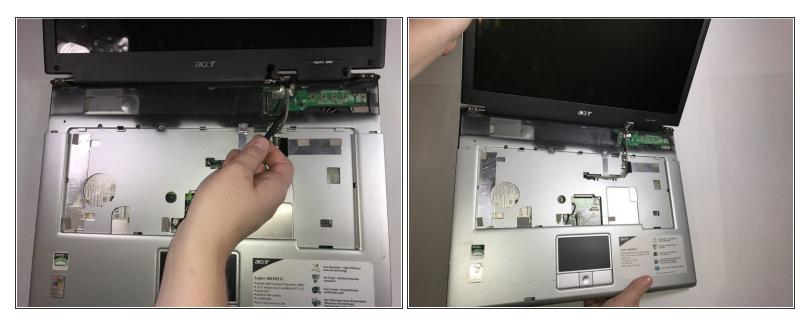
• Using a spudger, free the grey cable from underneath the plastic bars holding it within the body of the laptop.
