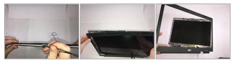
• After the bottom has been freed and the side of the casing has started to separate, one's hands can be used safely to pry apart the rest of the casing.
