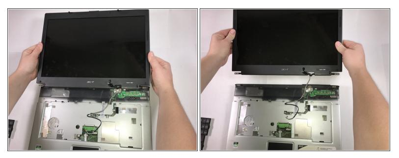
• Lift the screen and its casing away from the laptop.
