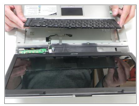
• Gently lift the top edge of the keyboard out of its place.
