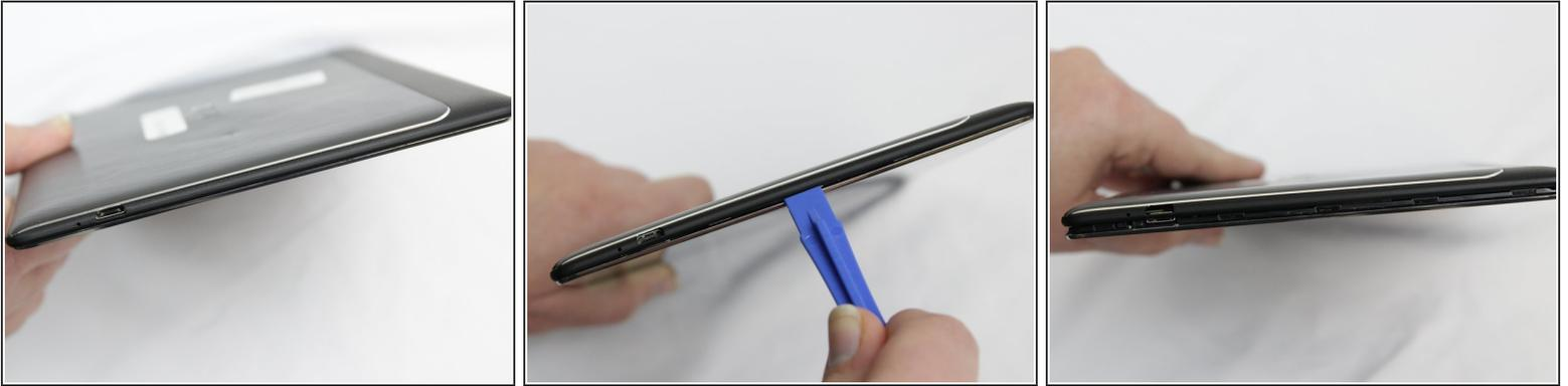
**⚠** if present, remove the MicroSD card before disassembly. Failure to remove could lead to damage to the MicroSD card, rear cover, or MicroSD card slot.
