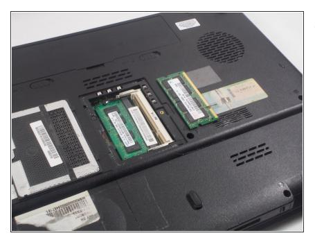
You should now be able to remove the first RAM stick by pulling it out in the direction of the long elevated side.
