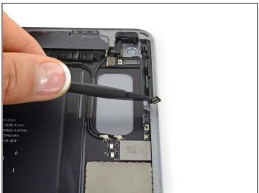
• Use the flat end of a spudger to pry up the volume button cable connector from its socket.
