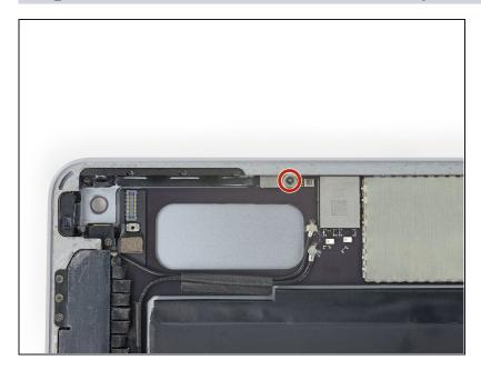
Remove the 1.2 mm Phillips screw from the bracket covering the volume button cable connector.
