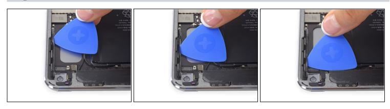
• Slide an opening pick underneath the volume button cable to break up the adhesive attaching it to the rear case.
