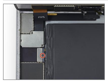
Remove the single 1.8 mm Phillips screw securing the battery terminals to their contacts on the logic board.
