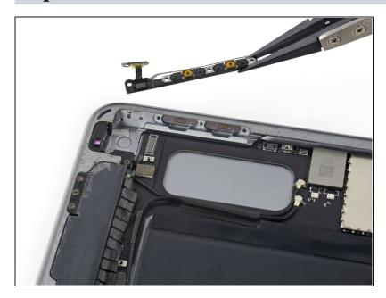
Remove the volume button and microphone assembly from the iPad.
