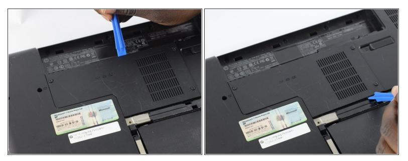
Using a plastic opening tool, insert it alongside any openings on the case. Lift and slide the tool to remove the case.
