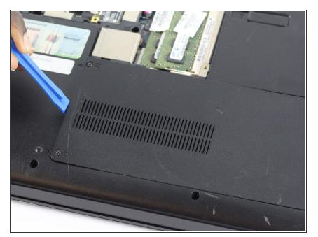
On the same side as the two screws, there should now be an opening to lift off the cover. Using a plastic opening tool, sightly lift the case up to remove it.
