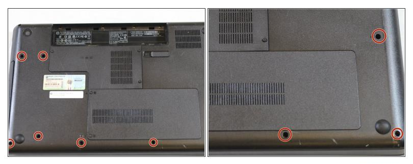
With all the screws removed from the previous guides. Remove the final eight M2.5X5 mm Philips screws on the back of the laptop
