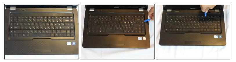
Open up the front of the laptop. Use a plastic opening tool to carefully pry open the keyboard from the edges.
