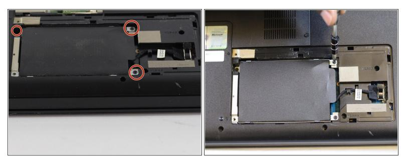
• Remove the three M2.5x5 mm Phillips screws securing the hard drive assembly.
