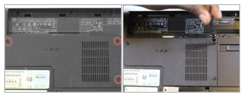
• Remove the three M2.5x5 mm Phillips screws securing the memory case.
