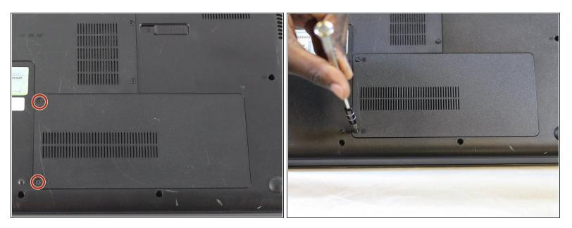
• Loosen the two M2.5x3 mm Phillips screws securing the hard drive cover.
