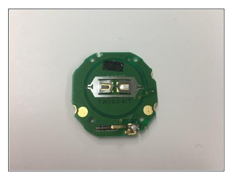
• Remove the battery by pulling from the sides to unstick the adhesive.
