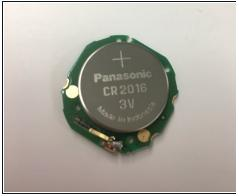
Remove the Battery Holder surrounding the circuitry of the watch by carefully pulling off each of the four clips.
