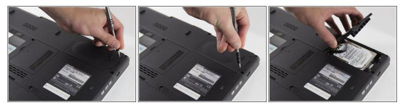
• Remove the panel that houses the storage drive by unscrewing the two 5.3 mm Phillips #1 screws that hold it into place
