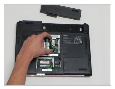
Remove the card by lifting up and away from the edge that has all of the contacts on it.
