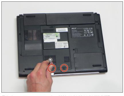
Remove the two 4.6 mm Phillips #1 screws on the lower edge of the laptop case.
