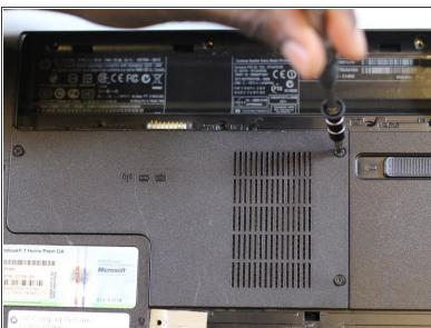
Remove the three M2.5x5 mm Phillips screws securing the memory case.
