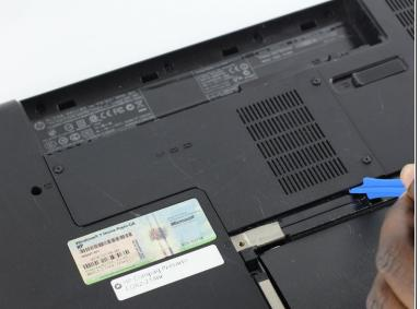
Using a plastic opening tool, insert it alongside any openings on the case. Lift and slide the tool to remove the case.
