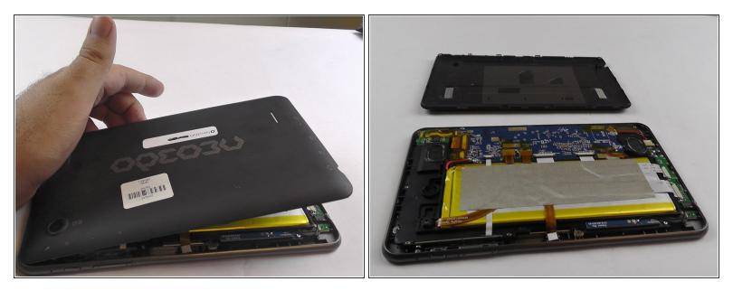
Once the back panel has been pried away from the bottom and sides of the Neo3DO, lift the back panel up and away from the tablet.
