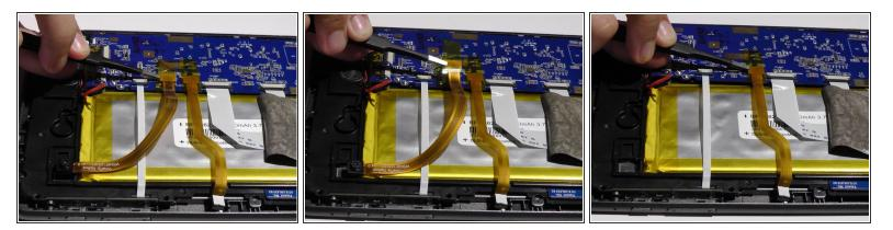
• Remove the ribbon wire from the socket.
