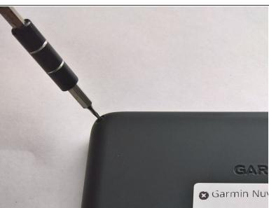
Using a T5 Torx Screwdriver, begin unscrewing the four 11.0 mm screws from the back panel.
